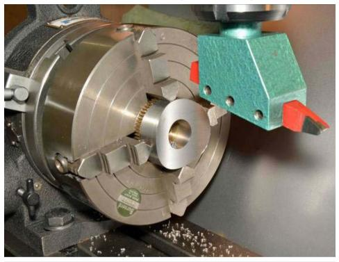
Photo 1: A substantial flycutter was used to finish the underside of a blank to suit the smokebox radius.
