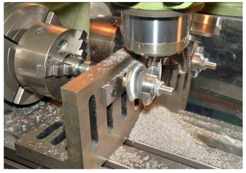
Above. Photo 2: The flared top surface of the chimney base was machined using a <sup>3</sup>/<sub>4</sub>in. HSS ripper cutter.
